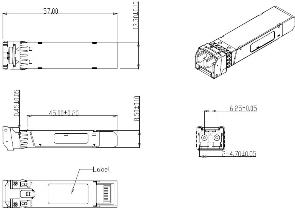
**Figure5. Mechanical Specifications**
